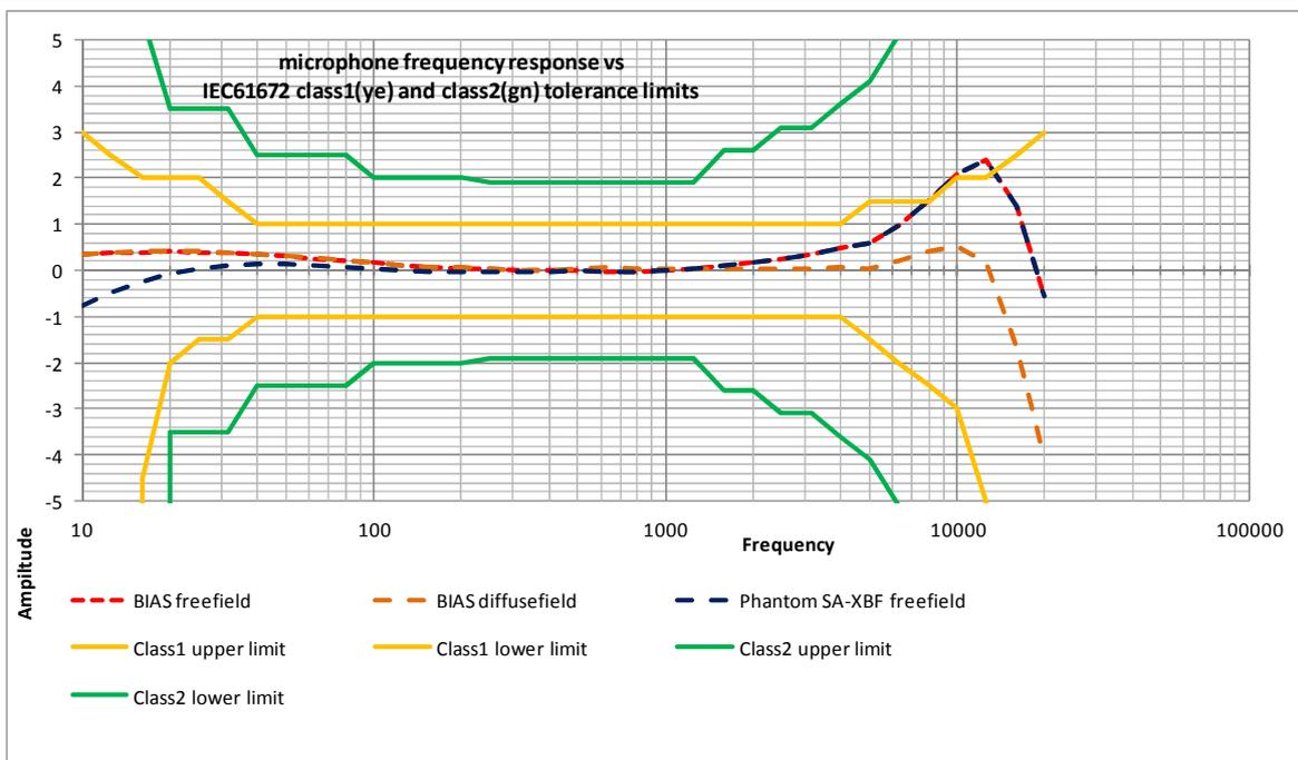
The diagram above shows the typical frequency response of an iSEMic 725TR microphone. Please note, that each microphone comes individually calibrated for free-field and diffusefield.
