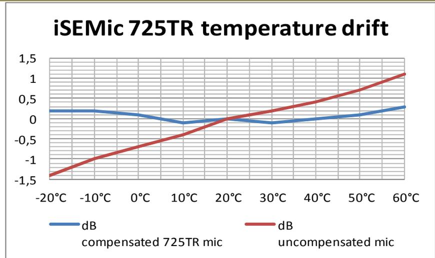
The range for the measurement was set at -20°C to 60°C which is more than iSEMcon microphones are normally used at. The most important temperatures are 10 °C up to about 50°C which covers indoor as well as open air use. It will give you a good predictable performance whether it is used in a cold autumn night or if the hot summer sun “burns” microphone body.
