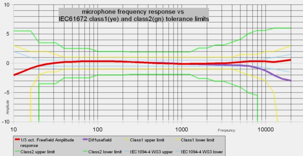
Microphone sensitivity: P48: 6,93      P24: 6,84      P12: 6,69      mV @ 94dBspl,1kHz
